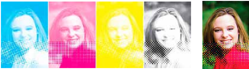
Cyan, magenta, yellow, and black (CMYK) separations with halftone exaggerated to show detail.
